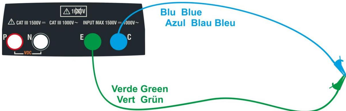
Fig. 4: Compensation of the measuring cables resistance
